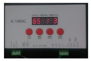
6. Please press and hold the "CHIP" key first, then press the "MODE" key at the same time to exit the addressing mode and enter the controller mode, as follow picture shows:
