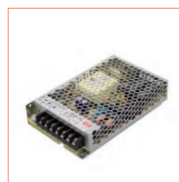
85-132VAC/170-264VAC by switch DC24V 150W IP20 Global certification Order Code: LRS-150-24
