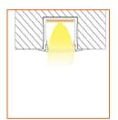
Name Straight alluminum channel Code BE1201 Material Alluminum Mounting style Recessed mounted Length Width 17.3mm Height 14.5mm Internal width 12.5mm
