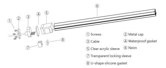
Step 1 Insert U-shape silicone gasket above the PCB board of neon.
